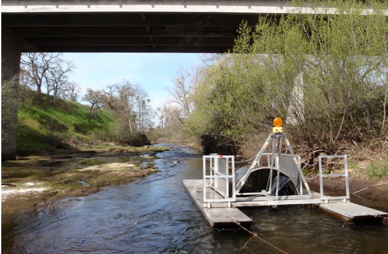
Figure 2. Five-foot diameter rotary screw trap operating during low flows on the Calaveras River at Shelton Road (picture taken on March 17, 2010).
