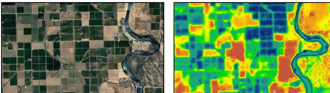
Figure 4 – Left: Landsat Image, Right: Calculated ET Image, at the instantaneous time of the satellite pass, 30m X 30m Pixel Sizes
